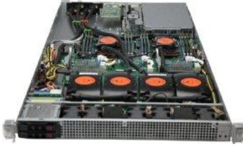
Figure 20: Direct-to-chip cooled rack
