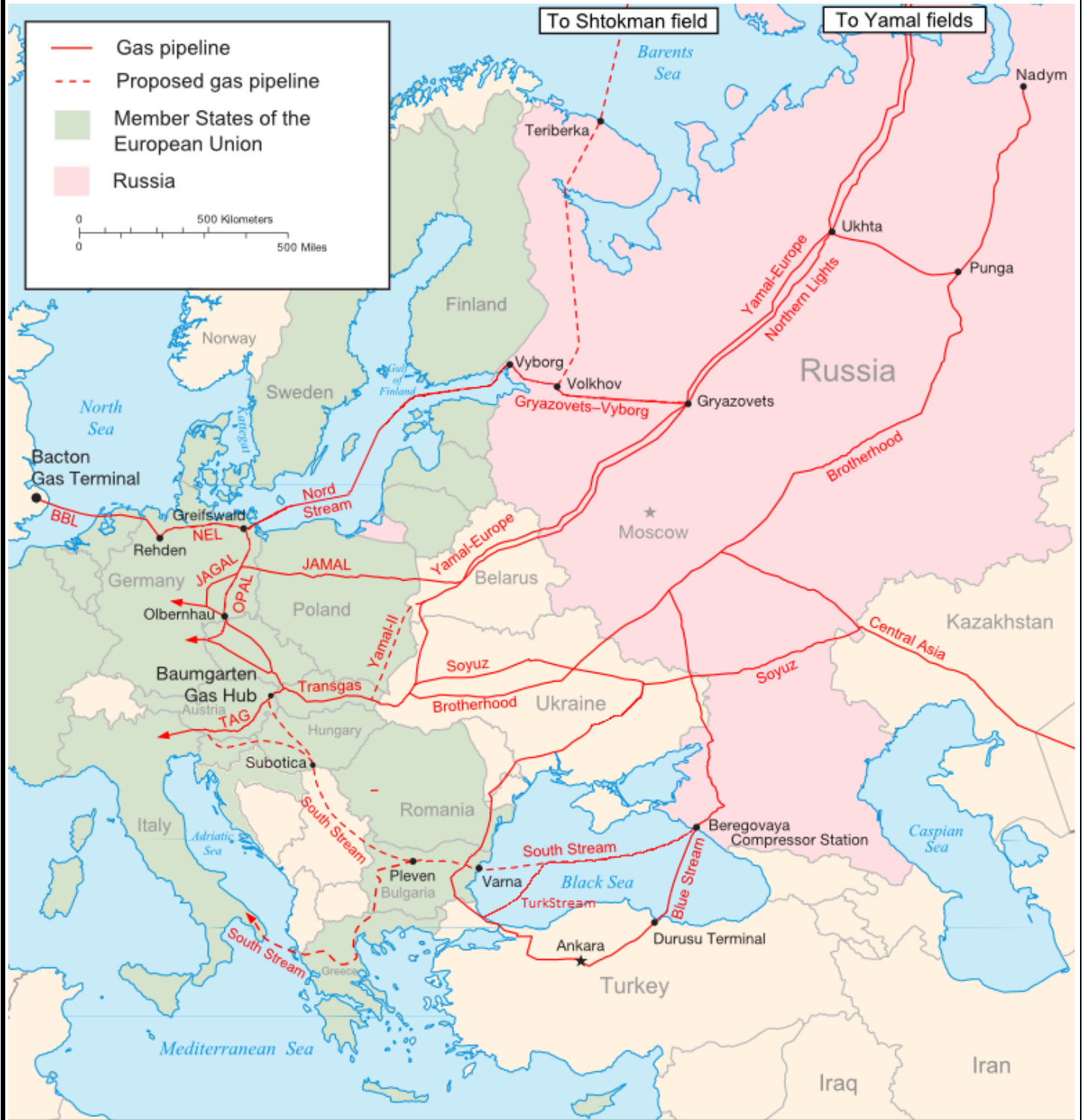
Figure 2: As of now, gas is supplied to Europe through three pipelines - Yamal-Europe, Nord Stream, Soyuz, and Brotherhood
