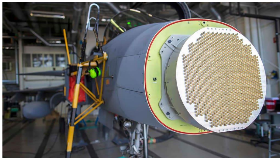
Figure 44: AESA radar, developed by BEL, is used in Rafale jets
