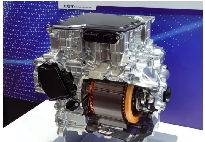
Figure 19: Aisin India's e-axle for Maruti Suzuki's eVitara
