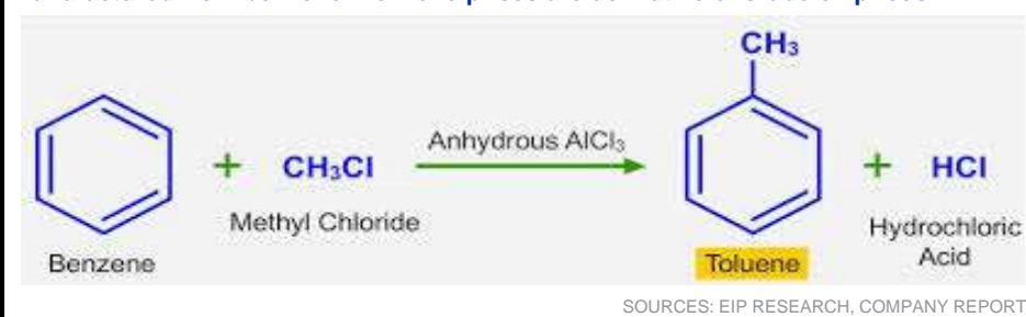
Figure 9: Toluene's price is determined by Benzene to some extent as Toluene is manufactured from benzene. Benzene prices are derivative of crude oil prices
