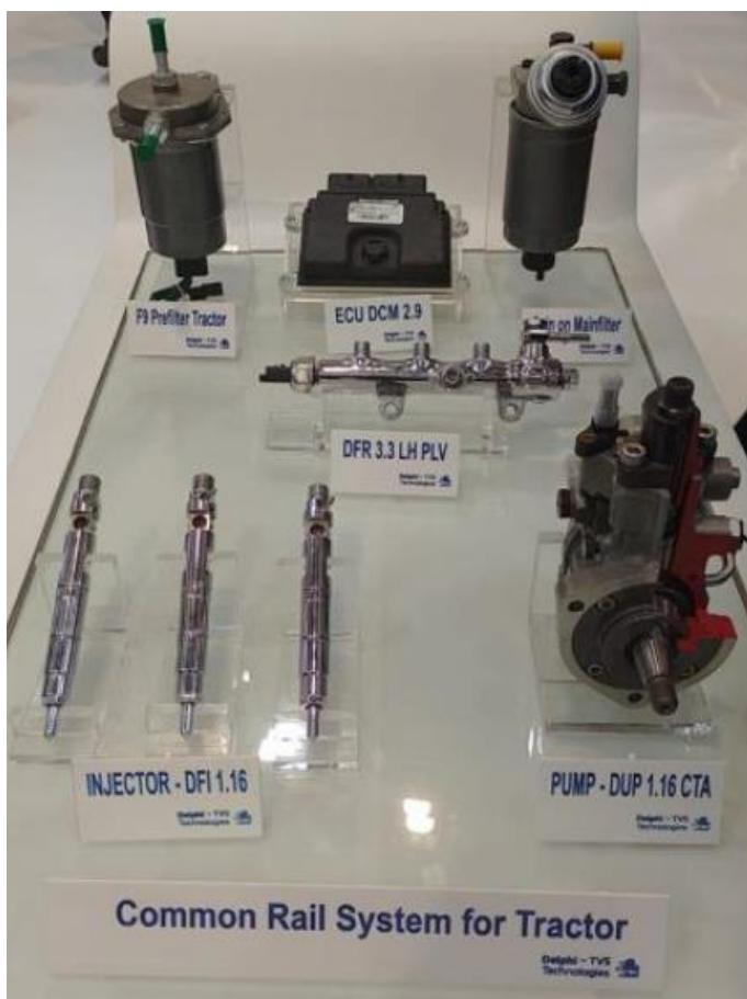
Figure 9: TVS Delphi product display of tractor parts to upgrade for meeting TREM-5 norms
