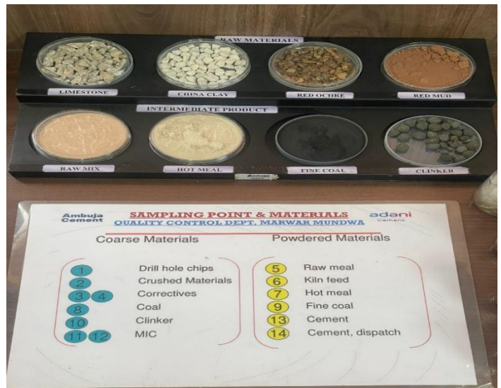
Figure 10: Sampling point for maintaining the quality of raw materials
